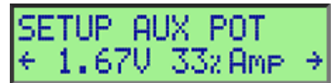
Live Vpot %Limit Mode Aux Pot with 3-position Switch and Current Throttle
