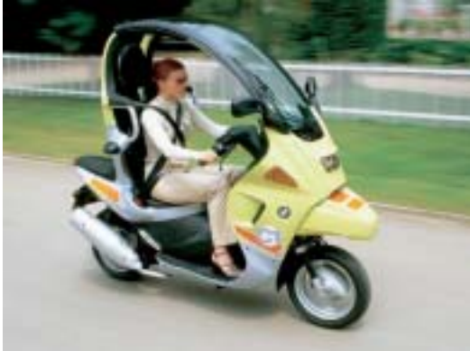
Figure 35: BMW C1: Motorcycle with roof, seat belts and no helmet, or just something completely new?
