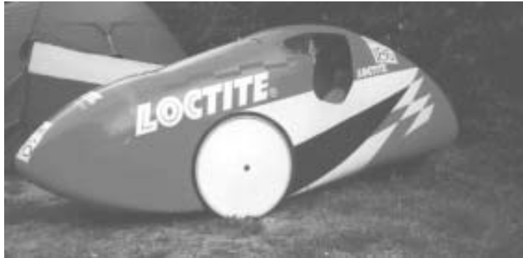
Figure 30: Windcheetah lightweight racing velomobile
