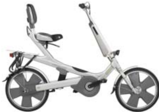
Figure 24: Giant Revive, an semi-recumbent bicycle, marketed on large scale (Picture from www.giant-bicycles.com )
