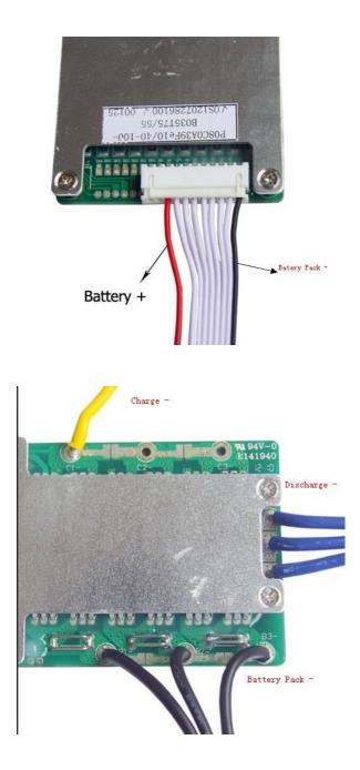
1. Connect the Balancing Wires: Please connect the black balancing wires from the battery's general negative
