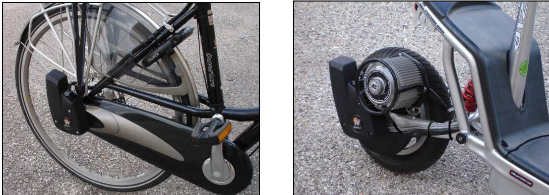
Figures 2 & 3: NuVinci CVP Developer Kit Bicycle (Batavus) and Light Electric Vehicle (Currie) Applications
