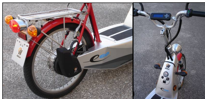
Figure 4: NuVinci CVP Developer Kit and NuVinci Display Interface Integrated Into a Light Electric Vehicle (eGo)
