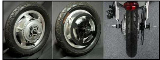
Figure 10: NuVinci CVP Housed in Rear Wheel
